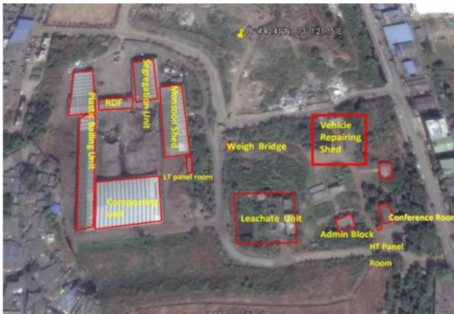
Fig.No.1: Satellite layout and schematic layout depicting sections at Turbhe landfill site
